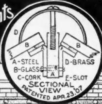
Handiest, Strongest and Most Practical Bar on the Market. Long Life—nothing to rot out. Glass Bedded on Spanish Cork, preventing cracking or Crushing of Glass. No putty, yet ABSOLUTELY WATER AND DUST PROOF.
