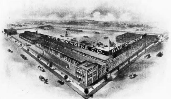
plant is equipped with machinery of the latest type, operates its own complete electric and water systems and private gas wells. Engines are built in sizes 2 to 100 h. p., in the stationary, portable, hoisting, pumping and electric lighting type. The plant has an output of 3,000 engines per annum. No other machinery is manufactured, being one of the few exclusive gas engine manufacturers of the country. Write today for catalogues, mentioning the AMERICAN CARPENTER AND BUILDER.
