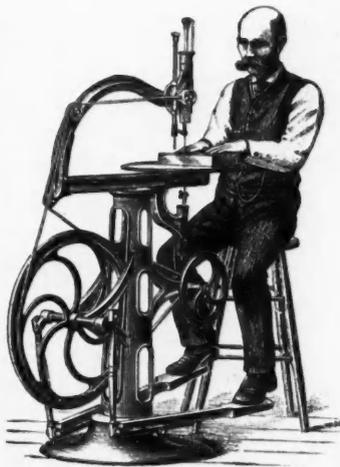
Suitable for carpenters, pattern and cabinet-makers and all wood-workers requiring accurate work, also for sawing soft metals. Will cut up to 3 inches thick, swings 24 inches, has powerful tread motion, cuts rapidly and is easy to operate. Has adjustable tension spring on upper spindle, dust blower, drill attachment, iron tilting-table, etc. Will furnish tight and loose pulleys for power in place of treadles when desired.
