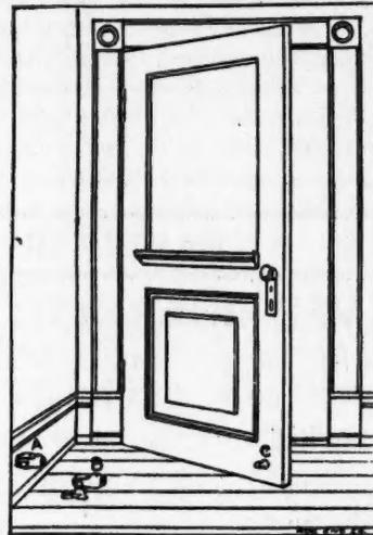
A—Swing stop attachment for base board. B—Showing stop attached to floor. C—Knob, which is always easily attached to door
