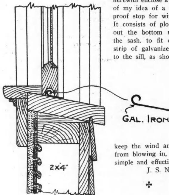
keep the wind and rain from blowing in, and is simple and effective.
