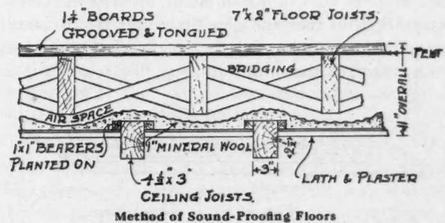
space giving perfect insulation, and also providing very desirable ventilation. Instead of the herring-bone strutting indicated, solid strutting might be used to advantage; but it would cost more.
