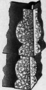
They are a neat and ornamental corner finishing, inexpensive and easily applied. These corners are made of 30 gauge galvanized iron, formed and punched with nail holes, ready to apply. There are two sizes—for four-inch and six-inch outside corners, also in both sizes for inside corners and octagons.
