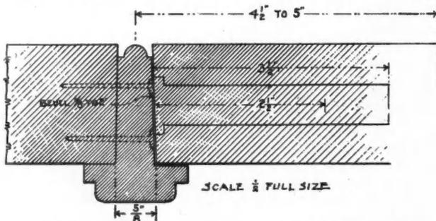
Detail No. 7. 1 1/2" Double Door on which Regular 3 1/2" Inside Lock is Used.
