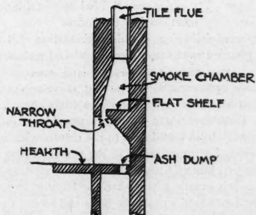
Sectional Detail Showing How to Construct a Smokeless Fireplace
