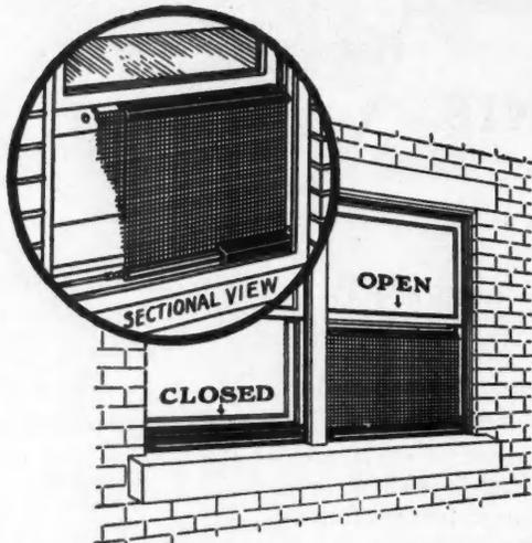
New Style Screen Works on Automatic Roller
