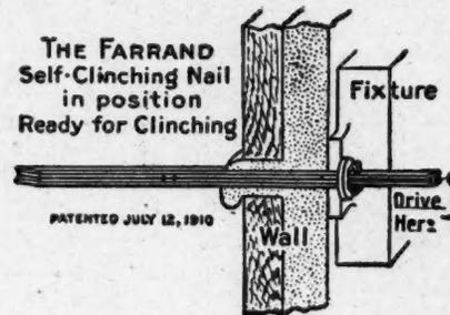
As shown in the first illustration, the top of the nail consist of a "driving stem" which protrudes through and above the washer-like head. This stem also extends down through the body of the nail, and is attached at its lower end to a couple of clinching prongs.
