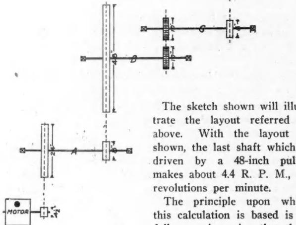
The sketch shown will illustrate the layout referred to above. With the layout as shown, the last shaft which is driven by a 48-inch pulley makes about 4.4 R. P. M., or, revolutions per minute.
