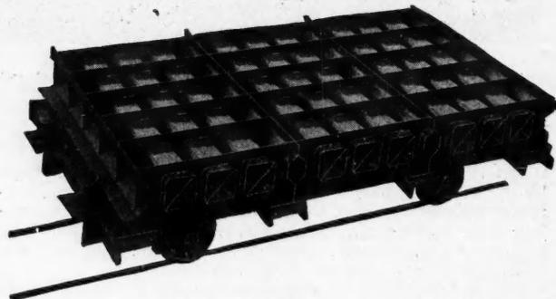
Set of Zagelmeyer Moulds Mounted on Iron Ball Bearing Truck
