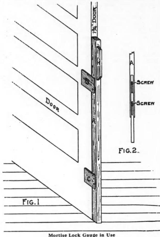
When the gauge is dropped to the floor, against the side of a door and given a light tap on "H," the nail points mark the centers of holes to be bored. No marking width of lock or gauging to the center of the door or anything else. Just tap your gauge and go to boring. I lay out my center line on "A" 7/8 inch from left side. When I get a 2-inch door I loosen the screws in "B" and slip in a shim 1/8 inch thick.
