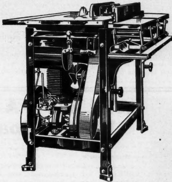
Showing Rip Saw and Jointer Attached
