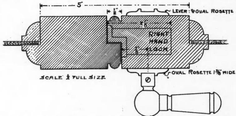
Detail No. 8. 1 1/2" Double French Window Having Rabbeted Lock, With Bit Key or Thumb Bolt
