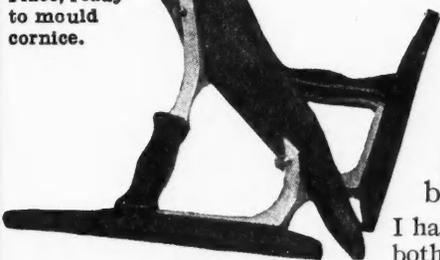
Showing Frame with Blade removed. Blades are easily changed.
