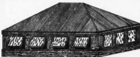
with swinging sash. Sides 24" high; all windows on each side made to open at the same time. Operating device locks them open or closed.
