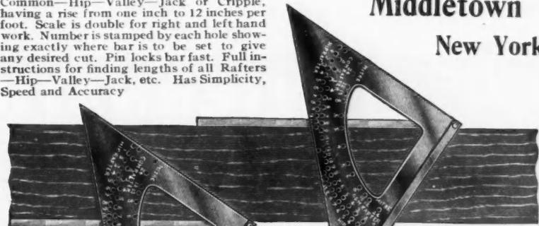
Showing Method of Cutting Plate and Ridge Cuts of Rafter.
