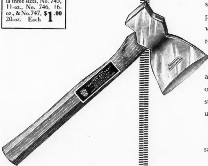
Famous Master-Builder Broad-Hatchet. Swelled bit throws chips and prevents wedging; rounded blade cuts at moment of contact. Octagon handle prevents slipping. No. 761, Size 1, & No. 762, \$1.25 Size 2. Each **1**
