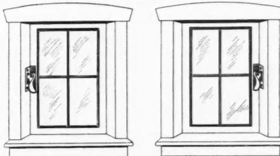
Recessed Casement Windows are Sometimes Trimmed with this Style Fast. These Fast are Made Handed and Very Often We See the Right Hand Placed on a Left Hand Sash and the Left Hand on a Right Hand Sash.
