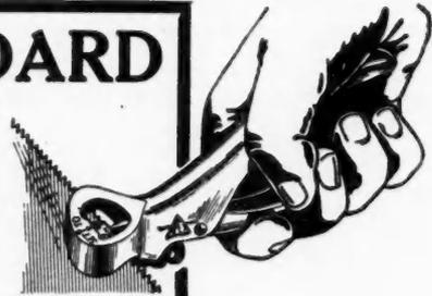
*The Morrill Special Saw Set* accurately sets any hand saw; takes out the wrong and puts in the right set at one operation. Send for Free Booklet: "Saw Points."
