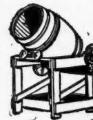
George C. Sheldon, Box 320-R, Nehawka, Neb., has overcome these faults by making a simple gear, pulley, and trunnions, and also some deflectors to be bolted inside the barrel. This equipment may be put on any stout barrel; and by making a frame of 2 by 4's and 2 by 6's, a man can have a mixer at a few dollars' expense, and two or three hours of work. The mixer may be run either by hand or with a small engine, and will mix 3 cubic feet of concrete at a time, dumping it into a wheelbarrow.
