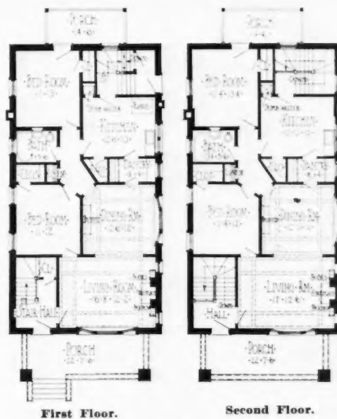
Arrangement of Interior of Three-Flat Building.
