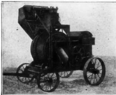
Wide loader and opening into drum permit fast charging without clogging.
