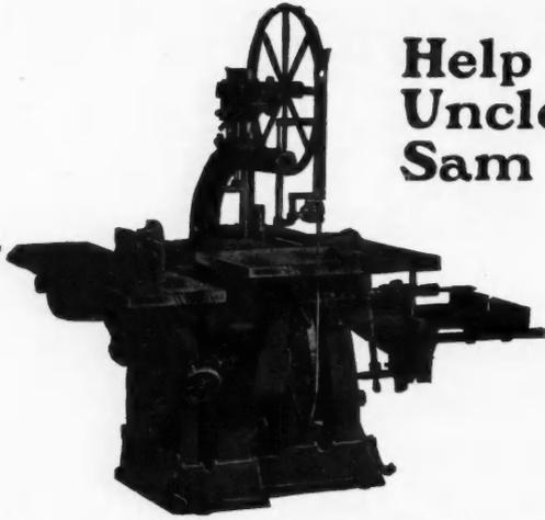
You can spare some of your men for government work by purchasing a Universal Woodworker. Now, of all times, is the time to increase the efficiency of your working force by employing this high grade woodworker for BAND SAWING, CROSS CUTTING, RIPPING, RE-SAWING, PANEL RAISING, GROOVING, DISC GRINDING, SANDING, JOINTING, BORING, TENONING, DADOING, KNIFE GRINDING and MORTISING.
