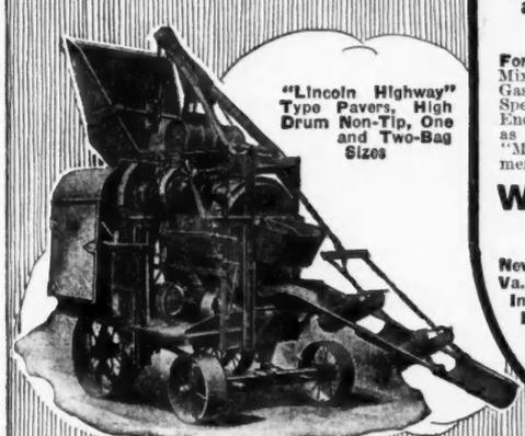
"Lincoln Highway" Type Pavers, High Drum Non-Tip, One and Two-Bag Sizes
