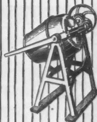
Showing Mixer unmounted in unloading position.
