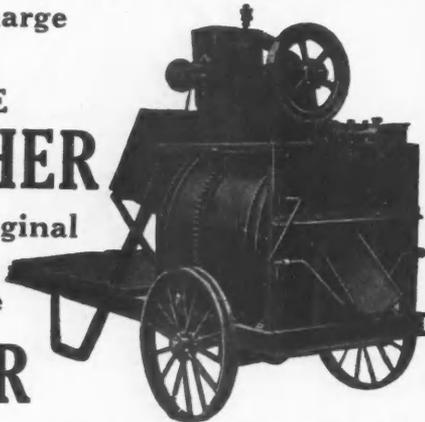
The end-discharge drum is mounted on a two wheeled truck and this means you can deliver the wet mix direct into the forms—no wheelers needed. No loading platforms to build and move away. Two men can move the ARCHER anywhere without the aid of a team.
