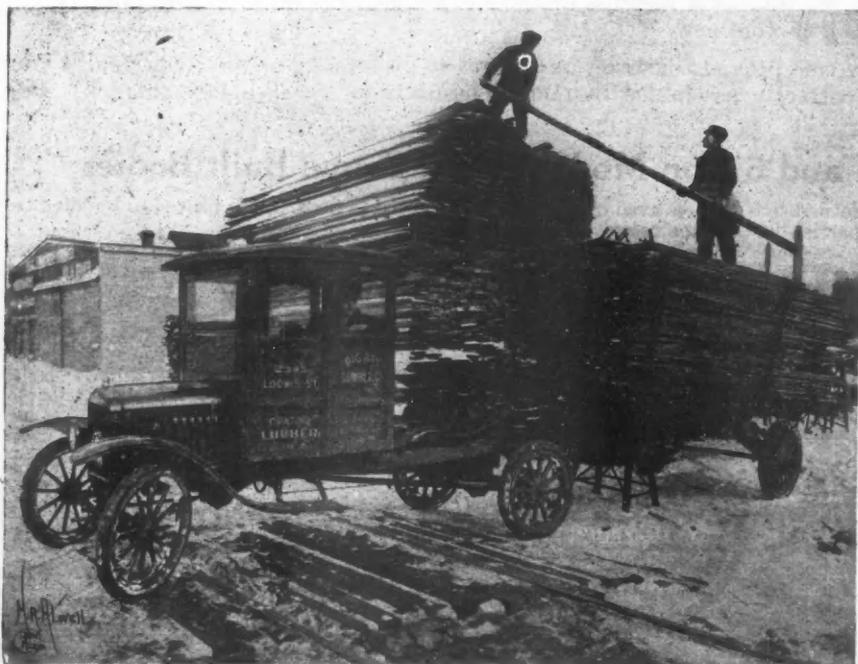
Loading Up a "Martin Rocking Fifth Wheel" Semi-Trailer with Lumber in the Big Bay Lumber Co.'s Chicago Yard. While One Trailer Is Being Loaded the Other Is Being Hauled to the Job.
