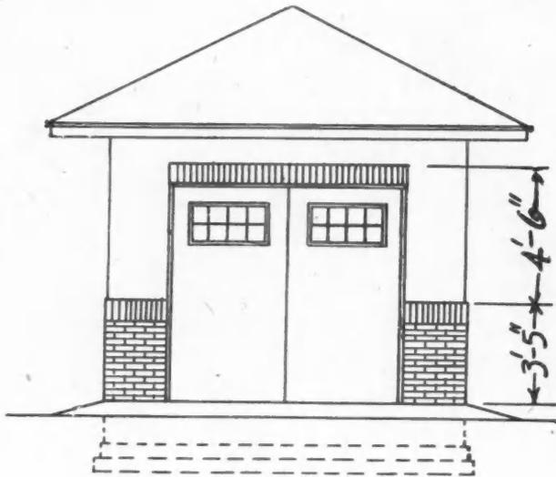
Front Elevation of Single Car Garage, 12 by 20 Feet. Constructed of Hollow Clay Tile with Brick Veneer on Lower Part and Stucco Above.
