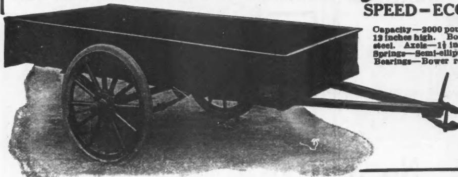
Capacity—2000 pounds. Body—8 feet long, 46 inches wide, 12 inches high. Body and under frame built of open hearth steel. Axles—1½ inch square bed, special high carbon steel. Springs—Semi-elliptic, oil tempered and double heat treated. Bearings—Bower roller. Wheels—1½ inch spoke, artillery type, second growth hickory. Tires—32x3, solid rubber. Weight—624 lbs.
