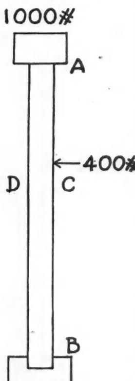
Figure 1. Showing a Post in Compression and Bending.
