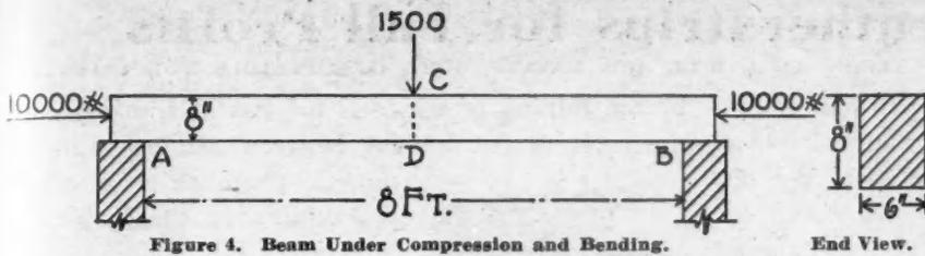
Figure 4. Beam Under Compression and Bending.
