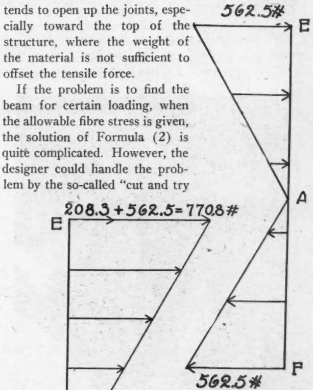
Figure 6. Bending Stresses.
