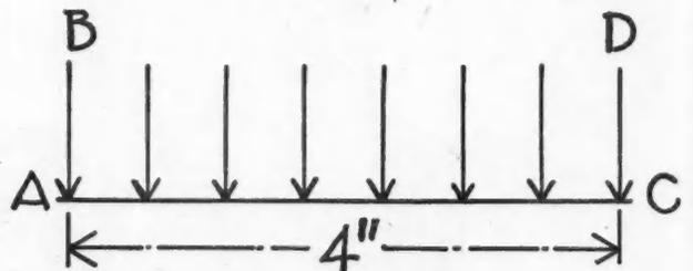
Figure 2. Representation of Uniformly Distributed Forces.
