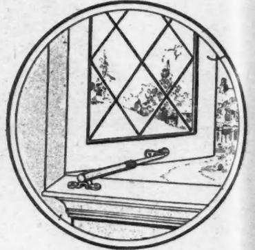
New Adjuster for Casement Windows Which Makes the Window Stay Put Wherever It Is Moved.
