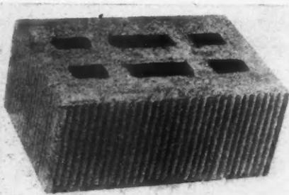
Figure 2. Concrete Structural Tile Made of Aggregate Under One-half Inch in Size, Showing Corrugated Surfaces Provided to Produce a Strong Bond with Stucco or Plaster.
