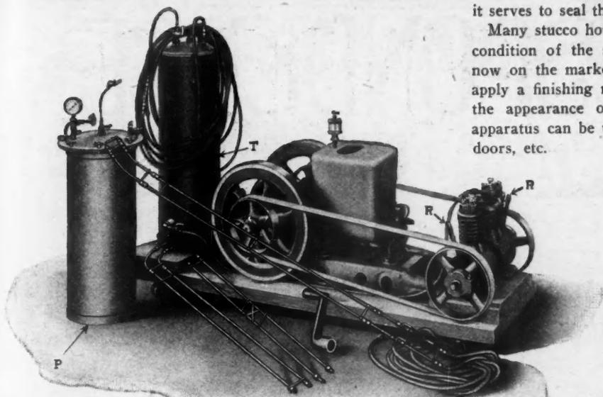
Complete Painting by Air Equipment Showing Engine, Paint Tank, Air Compressor, Rubber Hosing and Gun Sections
