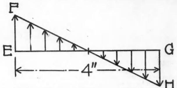
Figure 3. Showing Fibre Stresses Due to Bending.
