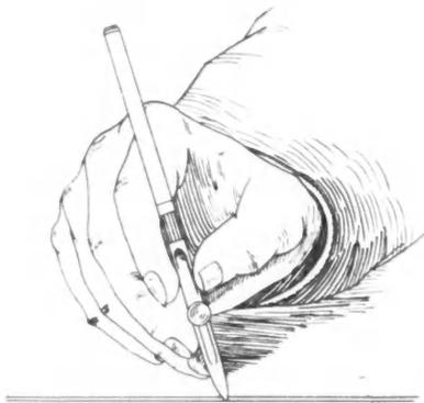
Fig. 7. Correct Method of Holding Ruling Pen.
