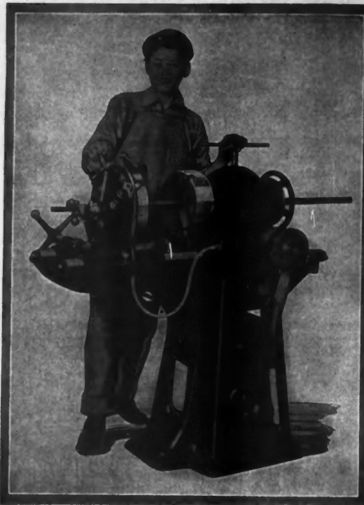
This Power Pipe Threading and Cutting Machine May Be Moved to the Work.
