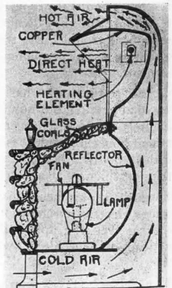
This Sketch Shows the Construction of the Electric Fireplace Heater.
