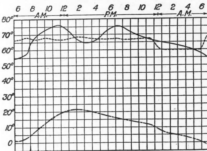
Fig. 1. Temperature Chart Showing the Result of Automatic Control Contrasted with Hand Firing in Domestic Heating. Solid line indicates hand firing temperatures, dotted line automatic control temperatures, lower broken line outside temperature.
