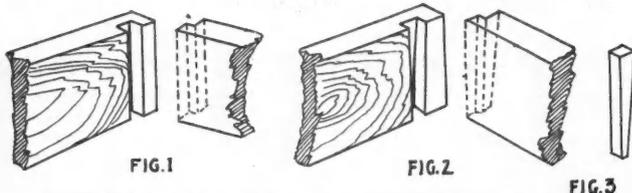
How the Baseboard Is Fitted with a Straight Dado or with a Tapering Dado Giving a Tight Fit and No Plaster Cracks.
