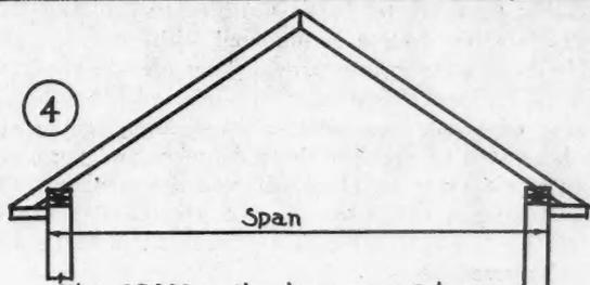
The SPAN is the horizontal distance covered by the roof, usually taken from outside to outside edge of plate
