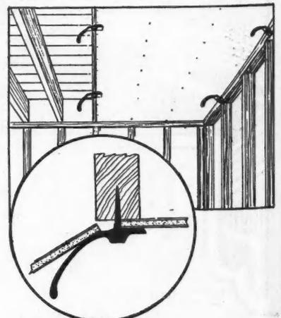
Both Time and Labor Are Saved in the Erection of Wallboard Ceilings by the Use of This Hanging Device.
