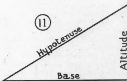
The RUN is the Base, The RISE is the Altitude, The LENGTH is the Hypotenuse
