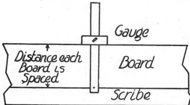
By Means of an Ordinary Wood Gauge, Siding Can Be Marked and Laid True and Straight Quite Rapidly Without Danger of Error.
