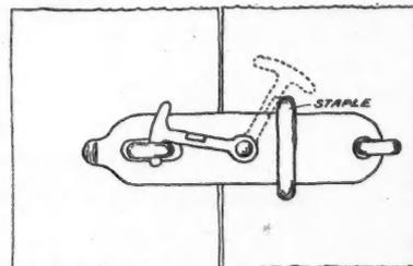
Convenience in Hooking the Hasp, Even When Carrying an Arm Load Is Possible by This Little Device.
