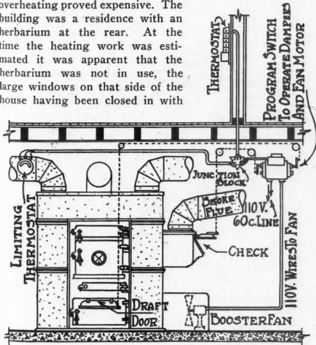
Fig. 2. One of Two Accepted Methods of Applying Thermostatic Regulators in Warm-Air Heating Systems, Showing the Dual Control.
