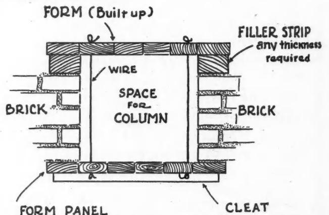
By This Plan the Brick Wall Is Built First and Serves as a Part of the Concrete Column Form.
