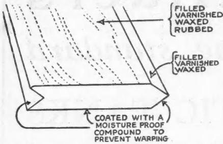
This Sketch Shows How the Ready Finished Flooring Is Treated to Prevent Warping.
