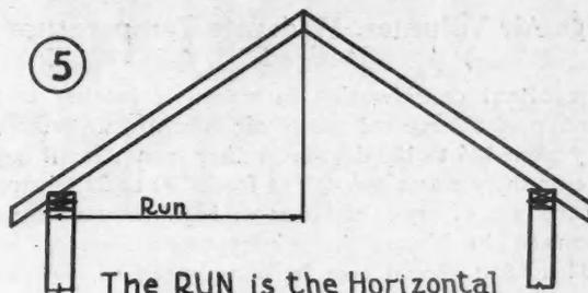
The RUN is the Horizontal distance covered by one rafter
