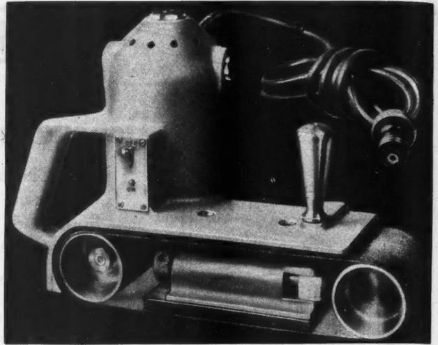
A Hand Sander Which Is the Latest of a Series of Machines Produced by a Leading Company in Its Development of the Electric Sander.
