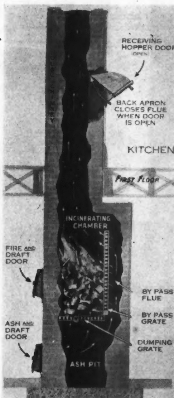
The Convenience of This Incinerator Can Be Appreciated by Looking at the Picture. Garbage, paper or refuse of any description can be instantly disposed of through the hopper doors at each floor above.
