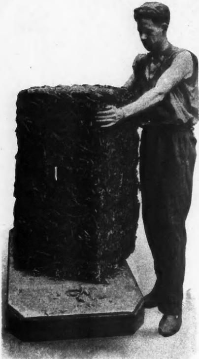
**Insulating Board Which Will Not Deteriorate, Crack, Warp or Buckle and Is Not Affected by Rain or Vibration, Is Made from the Licorice Roots Shown in This Bale.**
