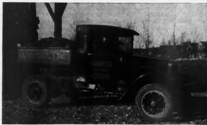
Wherever you go you will find International Model SD Dump Trucks rendering profitable service for builders. This view shows an SD-46 owned by A. G. Baxter of Calgary, Alberta, Canada. Every day it hauls from 45 to 60 yards of washed gravel swept out of the Bow River.
