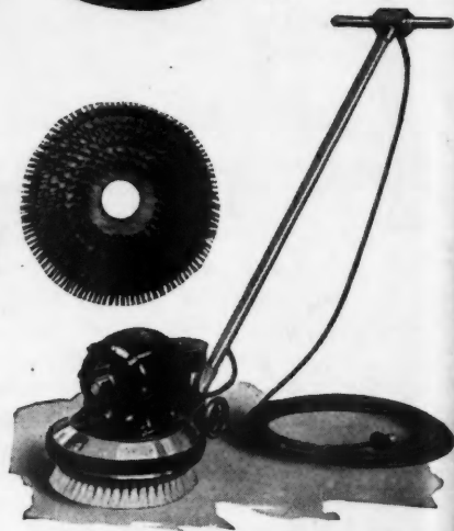
This Simple Floor Machine Is Suitable for Scrubbing, Polishing and Removing Varnish. The insert at the upper left shows the various brushes used.
