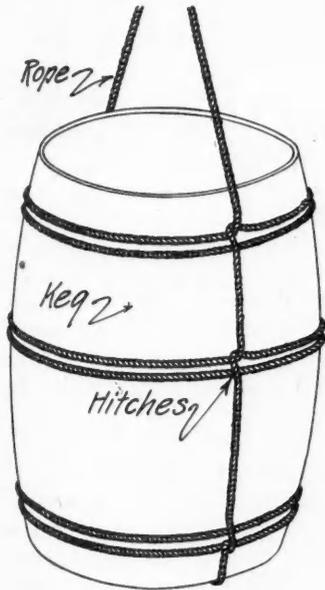
The Barrel-Hitch, for Hoisting Broken Nail Kegs.
