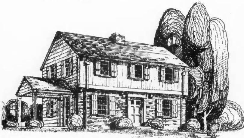
Exterior Walls: Wood siding exposed 8½ to the weather on side and rear walls, building paper, shiplap on 2 x 4 studs 16 o.c., plaster on wood lath; 4 brick veneer on lower half front wall; vertical siding on upper half front wall.
