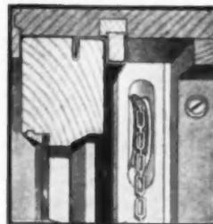
True counterbalancing insures a lifetime of trouble-free sash operation. Flat weights allow for narrow trim.
