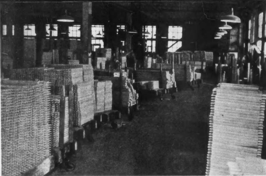
LEFT, UPPER: Stiles and rails ready to go to the door-drivers or set-up men. Some door factories can assemble more than 5,000 stock doors a day. LOWER: The durable construction and excellent finish of stock doors are made possible by advanced design and the use of modern equipment; part of which is this huge battery of 8-drum, motor-driven sanders.
