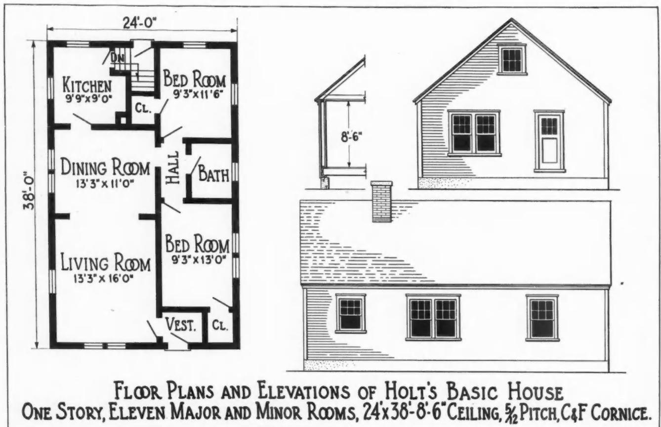
FLOOR PLANS AND ELEVATIONS OF HOLT'S BASIC HOUSE
