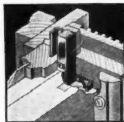
Section through jamb showing Andersen double action Silver-Seal Weatherstrip. Has both rib and spring metal contact and frictionless surface.
