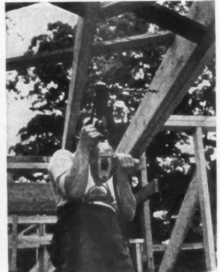
ANGLE DRIVE ATTACHMENT simplifies boring of holes in many hard-to-reach places.
