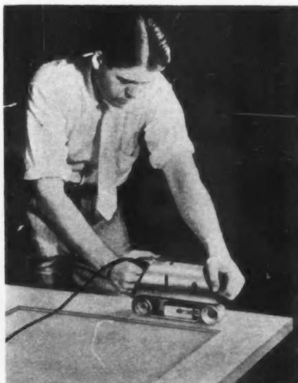
**BELT SANDER** does a fast job of surfacing and refinishing on wood or other materials.
