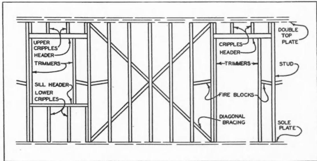
BASIS for determining lengths of standard framing members is indicated in this sketch, used in connection with formula described in accompanying article. Lengths of stud and header are guiding factors.
