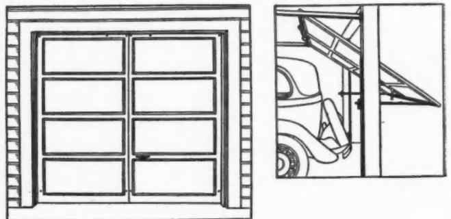
DIAGRAM showing front view and method of operation of the one-piece Craw. Fir-Door, a popular up and over model.
