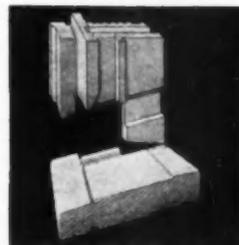
Locked Sill Joint is leakproof. Steep sill slope and chamfered blind stop insure quick drainage.
