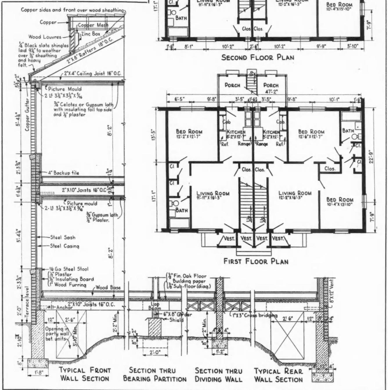
TYPICAL SECTION above shows brick and tile walls, frame construction, air space under first floor with passage between units, steel window casings, termite shields. TYPICAL FLOOR PLAN shows 3 and 4-room apartments, each with own front entrance and individual back porch and stairs. Above plan, used in reverse and with minor variations, was used throughout project.
