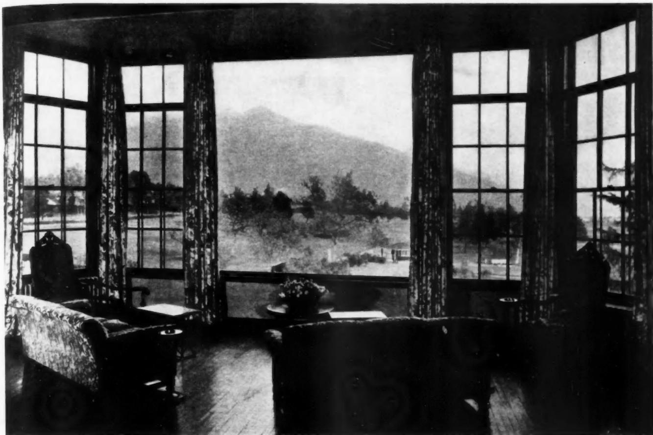
IMPROVED WINDOWS with "Aklo" plate glass that absorbs heat while transmitting ample light. This photograph shows a picture window in a California residence. The sun's heat rays are stopped while the shorter light rays pass through.
