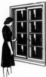
TO OPEN: Unlock and push sash outward and to right.
