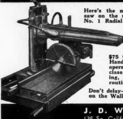
Here's the most practical contractor's saw on the market today—the Wallace No. 1 Radial Saw. With the exclusive Wallace Angulator, it cuts rafters complete with only ONE handling and without marking. It's a real money-maker on framing work, saving \$75 to \$200 on average homes. Handles every kind of sawing operation, and also does first-class shaping, dadoing, ploughing, grooving, fluting, bevelling, routing, etc.
