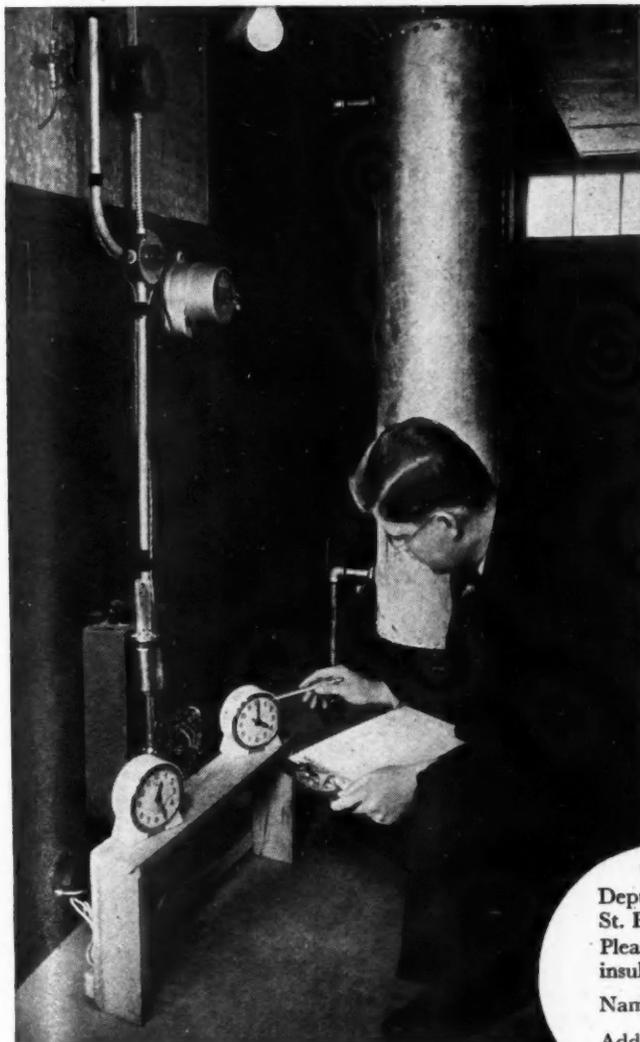
Checking time elapsed for various stages of fire during test period
