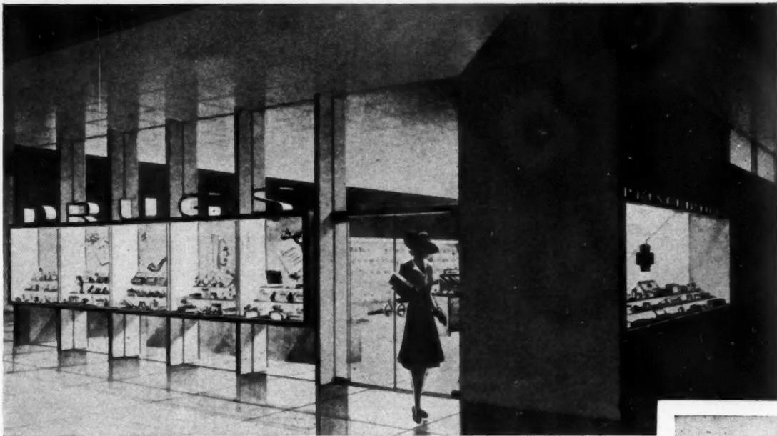
THIS perspective shows the corner of the drug store in the five-shop plan below. It has a protecting marquee in the form of projecting reinforced concrete roof slab, that shelters the varied ic-bies. (See side elevation.) Window display units are set between the vertical pre-cast stone slabs and are fluorescent lighted as detailed below. The balance of the store front is glass, including the entrance doors. Designed by M. Righton Swicegood, New York City.
