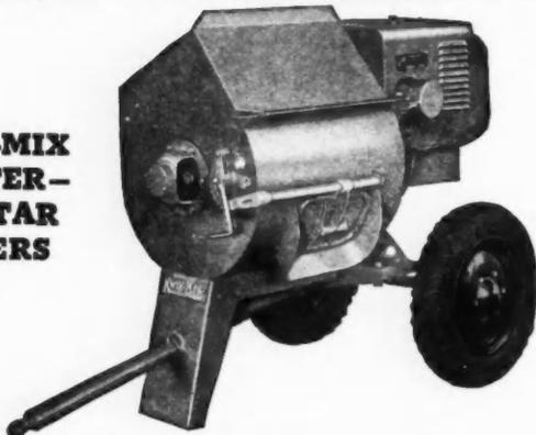
Kwik-Mix Non-Tilting 6-P Plaster or Mortar Mixer . . . fast discharge, 7 seconds . . . light weight, only 850 pounds . . . air cooled engine . . . V-belt and worm drive . . . low shoveling height. Also 4 wheel 10-P tilting model.
