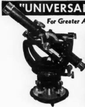
Especially designed for running levels and taking vertical angles on all survey and check-up operations... Patented Ball Bearing Race assures perfect adjustment under severest conditions... 25 power telescope... light, easy to operate... features of higher priced models. Write today for full information, prices and FREE booklet, "How to Lay Out Building Lots."
