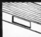
7" from top, 11" from bottom. Standard butt on 1<sup>3</sup>/<sub>8</sub>" doors, 3<sup>1</sup>/<sub>2</sub>"x3<sup>1</sup>/<sub>2</sub>"; on 1<sup>3</sup>/<sub>4</sub>" doors, 4"x4". Square corners. Center gaining for heavy construction is equi-distant between.
