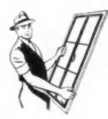
Installation of the Mesker "American Home" Metal Window is a time-saving, five minute job with hammer and nails. Just three easy steps . . . plumb, wedge and nail. It is adaptable for frame construction, for brick or for brick-veneer. And
