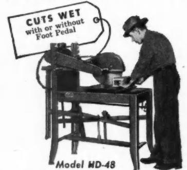
**DUSTLESS MASONRY CUTTING** so fast and easy. Just turn on the circulating water system and slice through the hardest masonry materials. Foot Pedal control for varying material sizes or lock the cutting head at a set position, whichever is desired.
