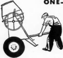
Here's the easiest handling tilter on the market. Rex Tele-pole towing tongue, easy-rolling pneumatic tires mounted with Timken bearings, plus accurate balance and light weight, make it easy for one man to spot the mixer . . . fast.
