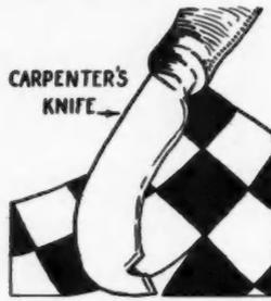
HERBERT E. FEY, New Braunfels, Texas, submits the above suggestion. Take an ordinary carpenter's knife and file a small notch in the inner edge near the tip. The notch must be filed sharp and clean. The notch prevents the knife from slipping when cutting linoleum. Circular cuts can also be made in this manner.
