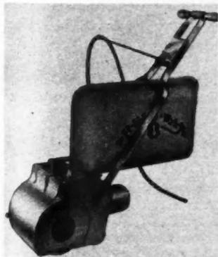
AB2817—The Reid-Way "8" Floor Sander, manufactured by Reid-Way, Inc. of Cedar Rapids, Iowa, makes use of an edger unnecessary in finishing floors. The sander works up to within one-half inch of the baseboard on both sides. The surface speed is 3,534 feet per minute and drum speed is 1,800 r.p.m. It weighs around 85 pounds.
