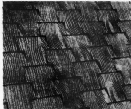
AB28139—An improved form of interlocking asphalt shingle called "Dubl-Coverage Tite-On" has been introduced by The Ruberoid Co., 500 Fifth Avenue, New York City, N.Y. A main feature of the design is an ingenious provision for overlapping which assures two thicknesses of shingle over every inch of roof deck and three thicknesses at vital points. The result is literally "two roofs in one." The shingles are made in a number of soft color tones.
