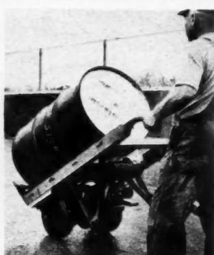
AB28177—The new Mototruk is made by the Comet Manufacturing Co., Minneapolis, Minn. It is built along lines of a conventional two-wheeled hand truck but with sturdier construction to accommodate heavier loads, and equipped with power to handle heavy work where there is no need for three or four-wheel trucks.
