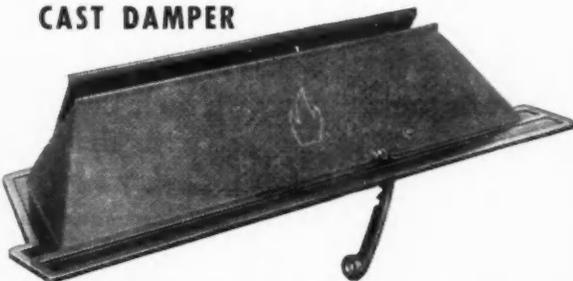
The Cast Damper with high dome, steep slope (50°). Steel valve avoids breakage. Broad, strong front flange may be used as lintel bar. These features, and sharp, clean lines make this the most up-to-date cast damper on today's market. The contractor's favorite cast-iron damper. Sizes 30", 36" and 42". Cat. No. C-103.
