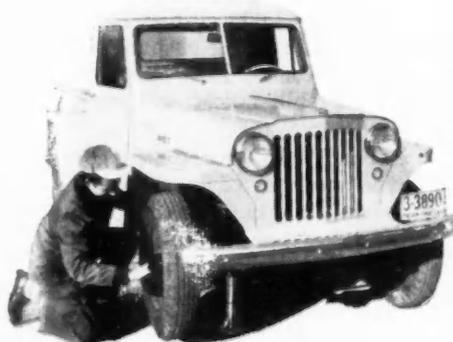
Flat, high-clearance fenders allow plenty of unobstructed room for quick tire changes. Fenders are hard to damage—and cost less to repair.
