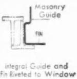
**2 EASY TO ERECT**—The masonry guide and fin make the window easy and inexpensive to install. Guide quickly aligns masonry. Fin ties window rigidly to construction.
