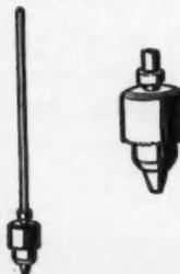
The standard spindle most commonly used with the drill press is the Jacobs chuck spindle in a 1/2-inch capacity. This is a key type chuck which grips the drilling tool firmly and evenly. This type spindle is used for most straight-shank drills or boring tools, and can also be used for sanding drums, plug cutters, machine spur bits, multi-spur bits, etc.
