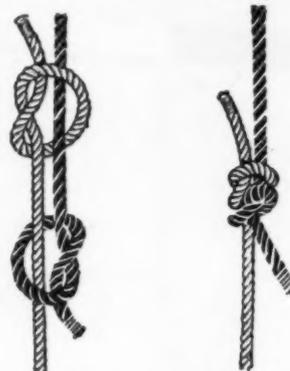
To tie: lay the two ends together—each pointing in the opposite direction. Then tie an overhand knot in the end of each—around the standing part of the other. When drawn tight, the two knots slide together and will not slip.
