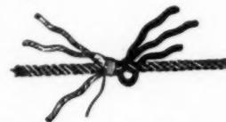
3. Tuck against the twist or "lay" of the rope. What happens is that the tuck goes over one strand, under the second, and out between the second and third.
