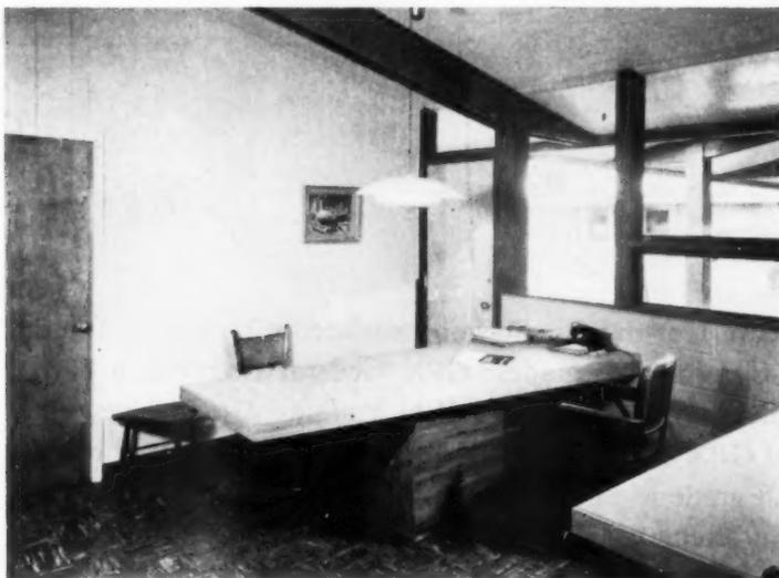
Wood office partition is used when it does not correspond to the beam module. Material is full 2-inch random width "V" jointed planking. Splines were used to eliminate shear action of the wood members. Builder claimed splines set in dado are easier to erect than using 2-inch 16g material
