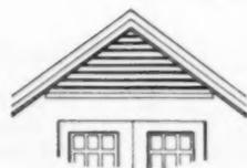
On new construction it costs little to include adequate exhaust openings for attic ventilation. These may be gable louvers or porch, soffit or basement exhausts, depending on the design of the house and individual preference.
