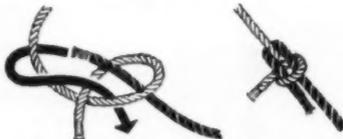
To tie: make an overhand loop with the end of one rope. Pass the end of the other rope through the loop thus formed, then up behind its standing part, then down through the loop again. Draw up tight.
