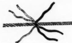
1. Unlay the strands of the ropes for a short distance, whip ends of the strands to prevent untwisting and put together as in diagram above, alternating the strands from each end.
