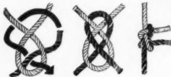
To tie: with one rope-end, form an underhand loop, so that both the free end and standing part point away from you. Start the second rope-end beneath both sides of the loop. Cross it over the standing part of the first rope, then under the free end of this first rope, and then over the left side of the loop. Cross it under itself and let the second free end lie over the right side of the loop. Finish by seizing each end to the standing part.
