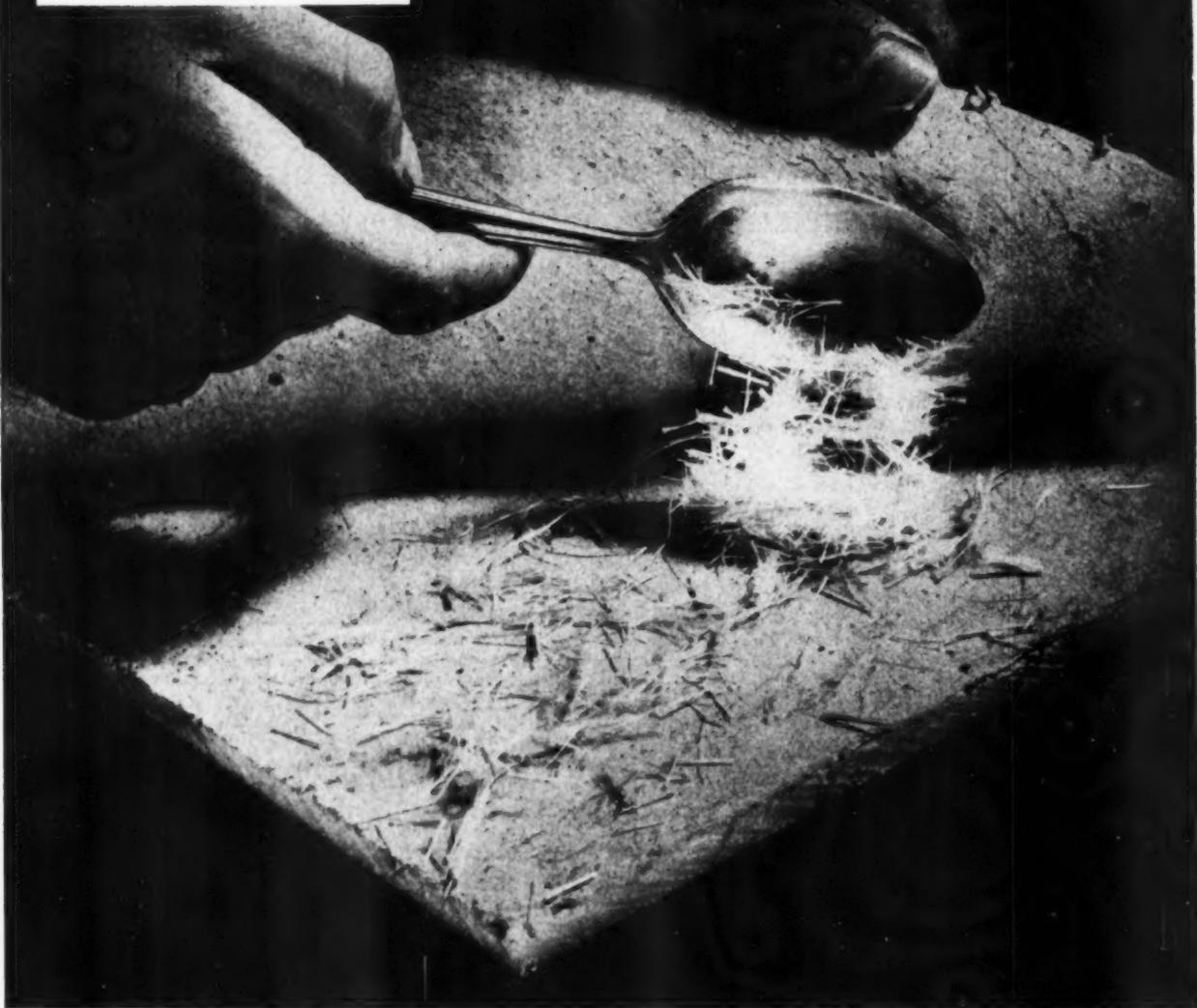
Mixing chopped Fiberglas yarns with gypsum plaster helps makers of gypsum wallboard to almost double the board's impact resistance!
