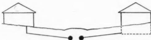
The ideal site takes advantage of natural drainage lines to keep sewer line connections at a minimum length
