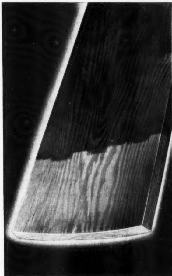
Paint can't protect improperly sealed wood from warping, swelling and blotching
