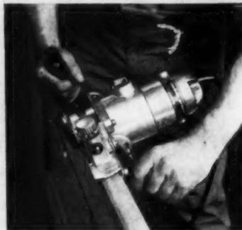
Plane cutter used in plane attachment. Will handle doors up to 1 1/2" in width. Leaves smooth, waveless surface that requires no sanding. Blows chips entirely free.
