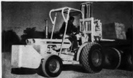
For higher, heavier materials-handling check this low-cost Case 430 Utility Fork Lift. It lifts 4000 lbs... works in mud, snow where small-wheel rigs mire. Hauls at high speeds, shuttle reverses instantly for fastest round-trips. Has many quick-change attachments for multiple specialized materials-handling work. CU-L-285
