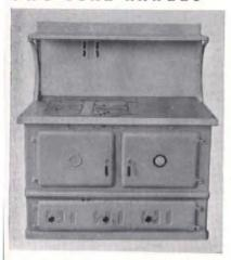
HEATERANGE. The Jeddo Highland Heaterange, to all appearances a coal burning cooking stove, is also a warm air furnace from which, by the usual arrangement of ducts, blower, and humidifier, warm humidified air is circulated throughout the house. As with other furnaces, a water back and storage tank provide for the supply of domestic hot water.
