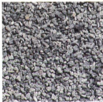
The basaltic gravel is manufactured with the specifically required size, shape and weight to form an effective barrier against the Formosan.
