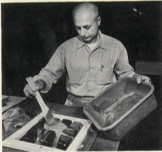
Filling in with cement (left)
