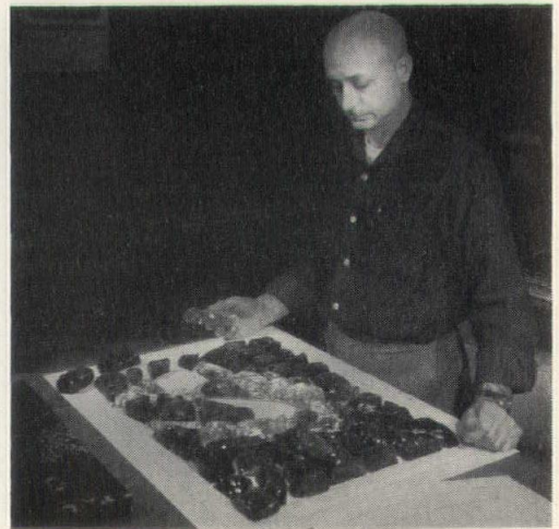
Shaping and placing glass to match color design (right)
