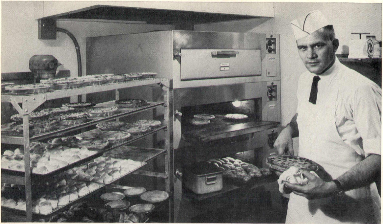
The kitchen in the Hobby Ranch House, Fort Wayne, Indiana. Notice the chef can bake potatoes or meat and pastries in the same electric unit at the same time. This gives the restaurant owner a big savings in time and labor.
