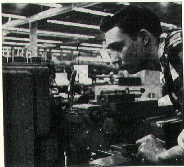
This is the central work area at Bowmar. The lighting system now provides 70 foot-candles illumination, and this will soon be increased to 110 foot-candles because of the experience in the testing and inspecting department.
