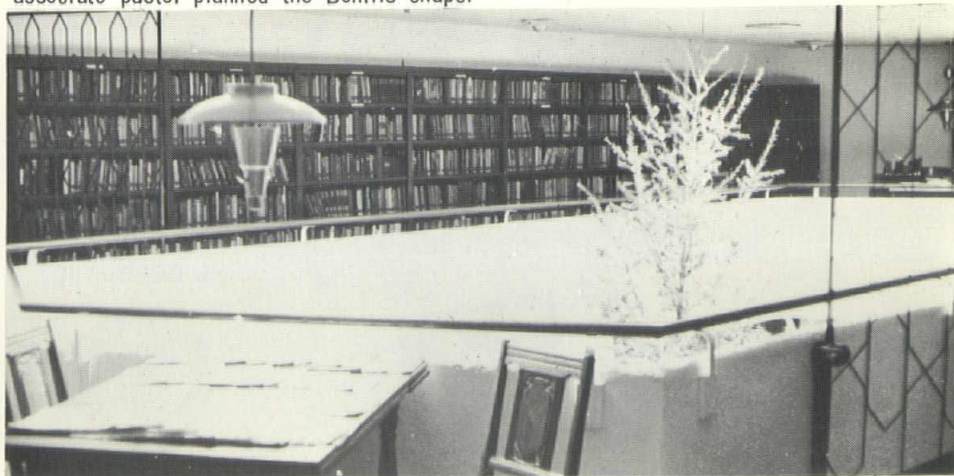
The church's library is on a mezzanine surrounding a light well. Low-cost sprayed concrete, now painted white, and steel framing were used throughout the church.
