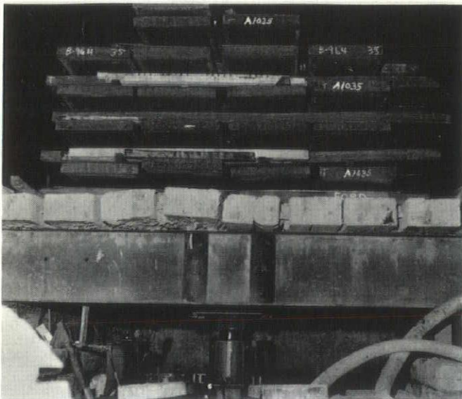
Pile, loaded with 250 tons of steel by Detroit Testing Laboratory engineers to verify its load supporting ability.
