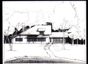
Private Cabin Lake Hubert, MN A low sloped roof to the north shelters and rises to the west and south to capture sun and lake view while directed views are placed in dormers above. The open loft and central living space gather around the anchoring stone fireplace. Designed by Wayne Branum.
