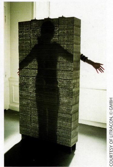
Herzog & de Meuron used a photoengraving technique to animate the bands of concrete panels that wrap the Eberswalde Technical School Library in Germany (above). The LiTraCon company markets translucent concrete blocks cast with optical glass fibers (right). These and other innovations are changing perceptions about concrete.
