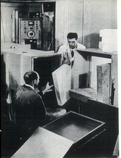
Architectural panel testing in Industrial Acoustics Company's new laboratory facilities in New York City: Transmission loss properties of a plastic foam sample will be tested when sample is sealed into duct at left. The two ducts will be connected and microphones placed on both sides of the test specimen to determine its acoustic transmission loss.
