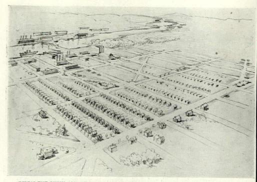
BIRD'S-EYE VIEW (CONVENTIONALIZED FOR COMPARISON) OF A TYPICAL COTTAGE DEVELOPMENT SHOWING THE LIMITED AIR SPACE AND GARDEN SPACE OBTAINED BY SUCH A LAYOUT.
