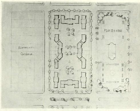
A TYPICAL PLAN OF ONE BLOCK OF TWO-STORY APARTMENTS INDICATING THE GREAT AIR SPACE PROVIDED BY THE METHOD OF HOUSING WORKERS.
