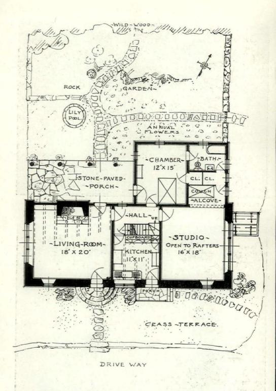
FIG. 6. FIRST FLOOR PLAN—COTTAGE OF MISS CAROLINE M. SPEARE, WOODSTOCK, ULSTER CO., N. Y. MYRON S. TELLER, ARCHITECT.
