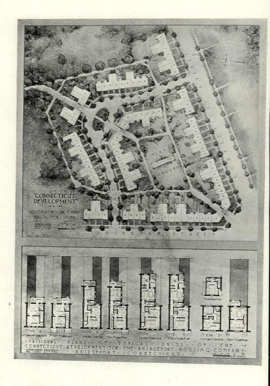
FIG. 34. GENERAL PLAN AND TYPE PLANS—BRIDGE-PORT HOUSING CO. DEVELOPMENT, BRIDGEPORT, CONN. SCHENCK & MEAD, ARCHITECTS.
