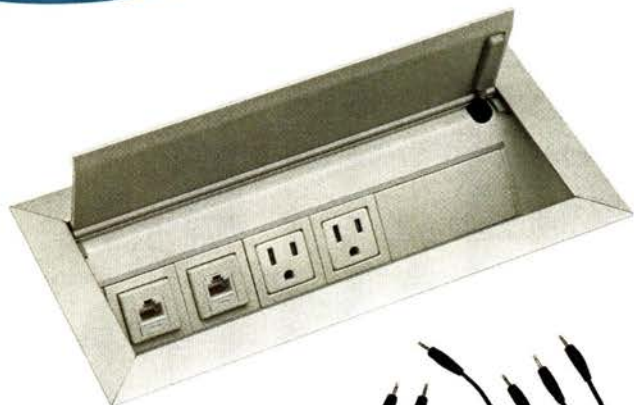
11 5/16" x 5 5/16" overall going into 11" x 5" cutout, has 6ft. cord. Finish: Satin Aluminum. UL listed.
