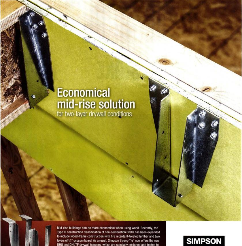
DHU and DHUTF drywall hangers, which are specially designed and tested to transfer floor joist loads to a wood stud wall through two layers of drywall. These hangers install after the drywall is in place so there's no need to cut around joists - making installation easier.
