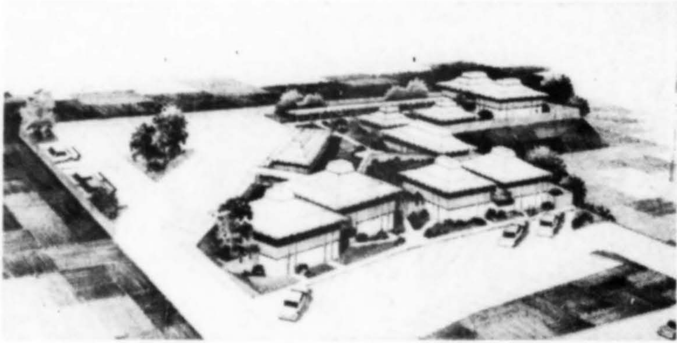
NORTH VALLEY VILLAGE medical-dental center, Thornton, Colorado, will have 10 buildings to be individually designed and developed for each tenant. The first major center of this nature in the area, each building will be masonry curtain wall, steel frame, wood framing for interior partition. Architects: Brelsford, Childress and Paulin, Denver.
