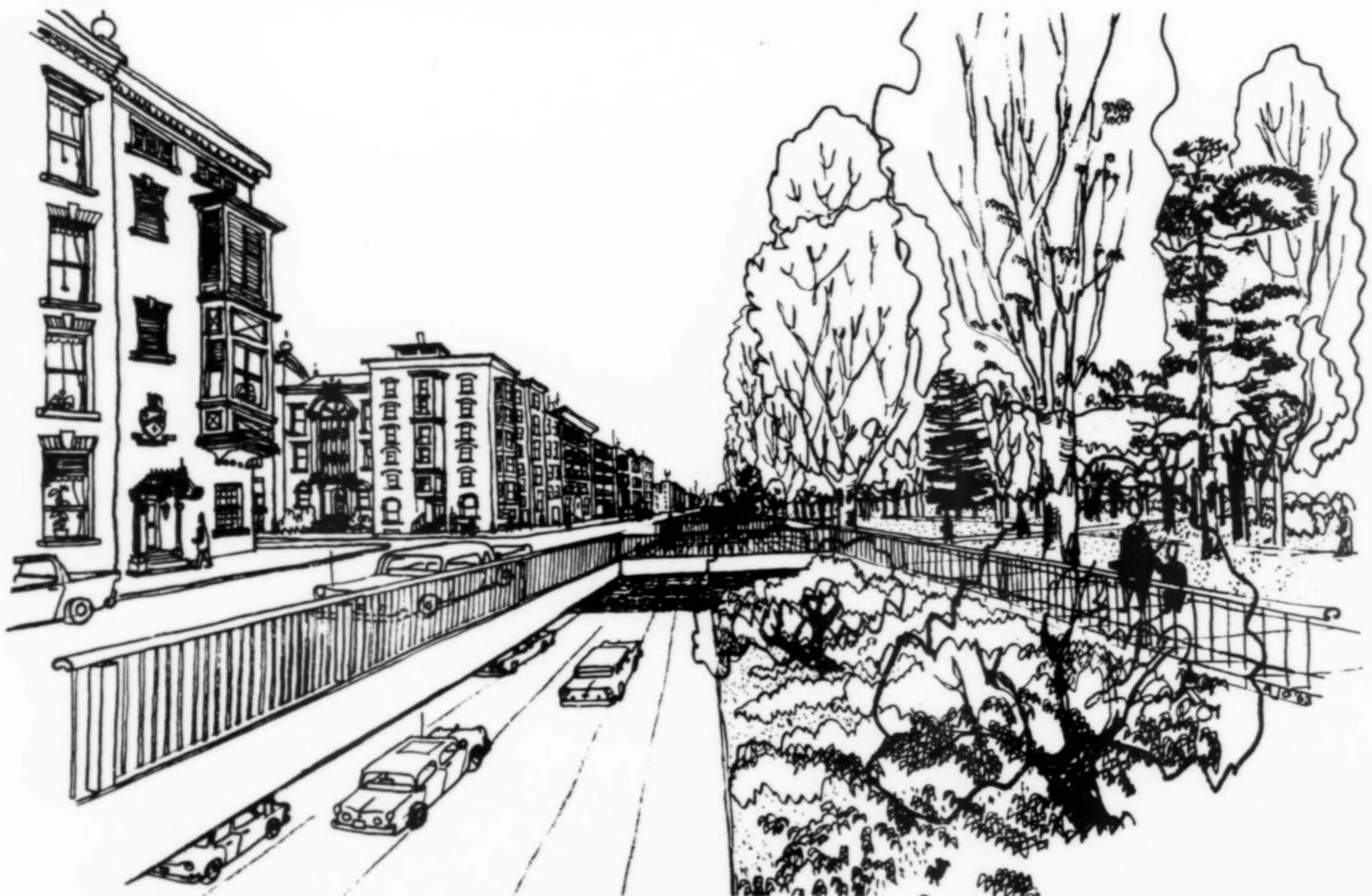
Local street cantilevered over depressed freeway.
