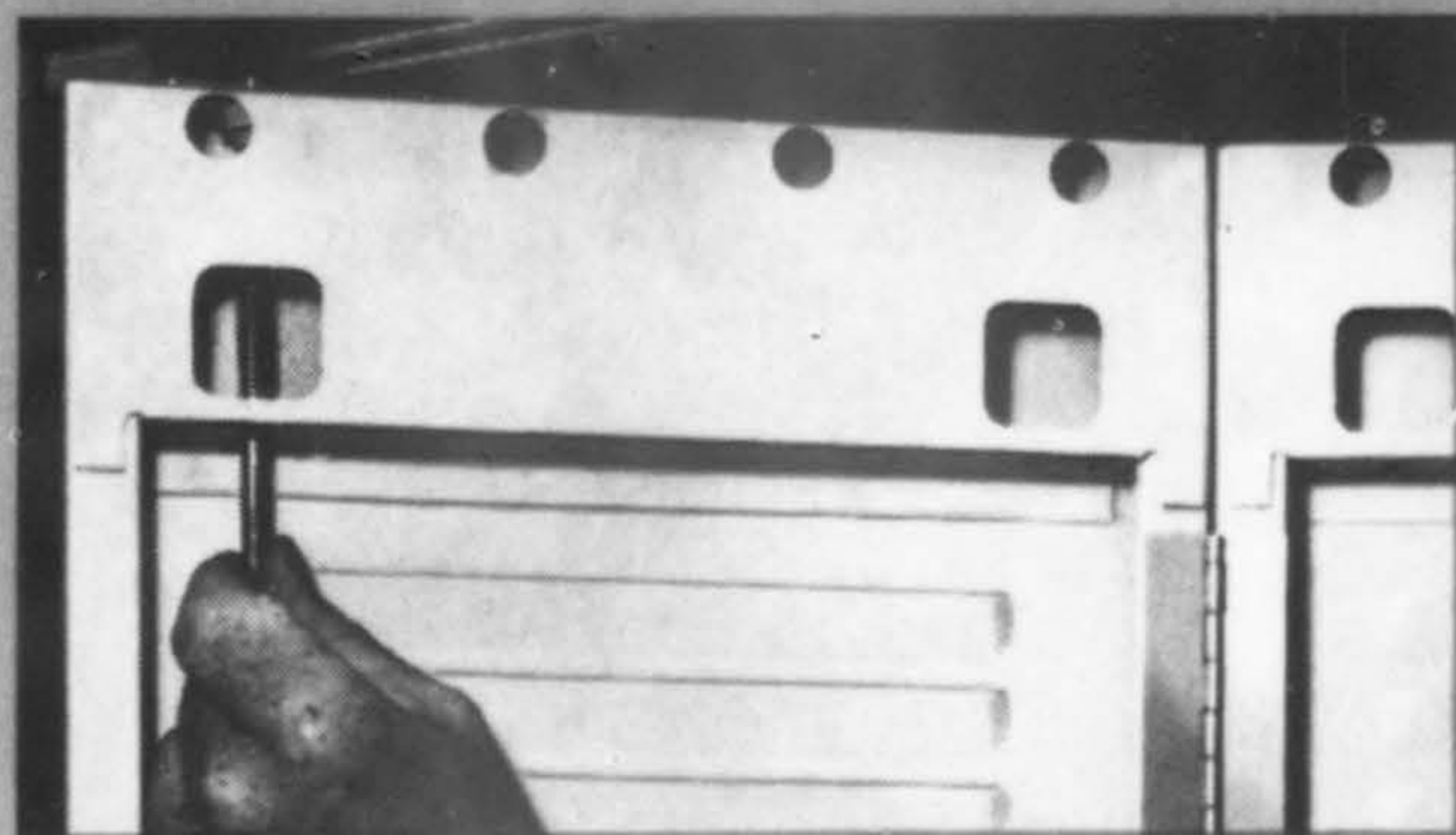
snap! upper pivot into upper pivot block.
