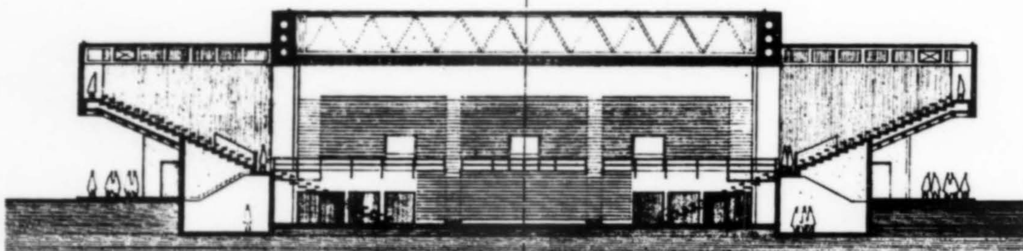
ROSCOE W. MAPLES PAVILION , Stanford University, will provide an indoor facility for overflow of cultural and educational events as well as athletic programs. An extra 2000 seats will be available by end-cantilevered sections to achieve a total seating capacity of 8000. Team rooms and public facilities will be under bleachers. Spectators will enter on the second level via stairways. Estimated cost: $2.16 million. Architect: John Carl Warnecke & Associates.
