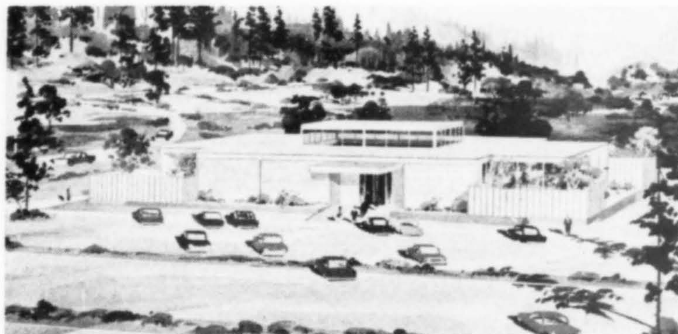
PUBLIC LIBRARY , Bellevue, Washington, will be a 18,500 sq. ft. structure, on one level, with provisions for a second level addition. It will be located on the Municipal Center site, just West of the existing Municipal Building. The steel frame building will have cavity wall brick panels on exterior. Cost: $363,000. Completion: November 1966. Architect: Ridenour & Cochran; Rudy Simone Construction Co., contractor.
